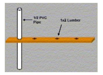
First take the PVC and cut it into (3) 32 in. pieces. Then drill (11) 5/8 in. holes along the length of the 1x2 studs, 8" on center. Now slip the pipe pieces into the holes in two of the 1x2 studs so
